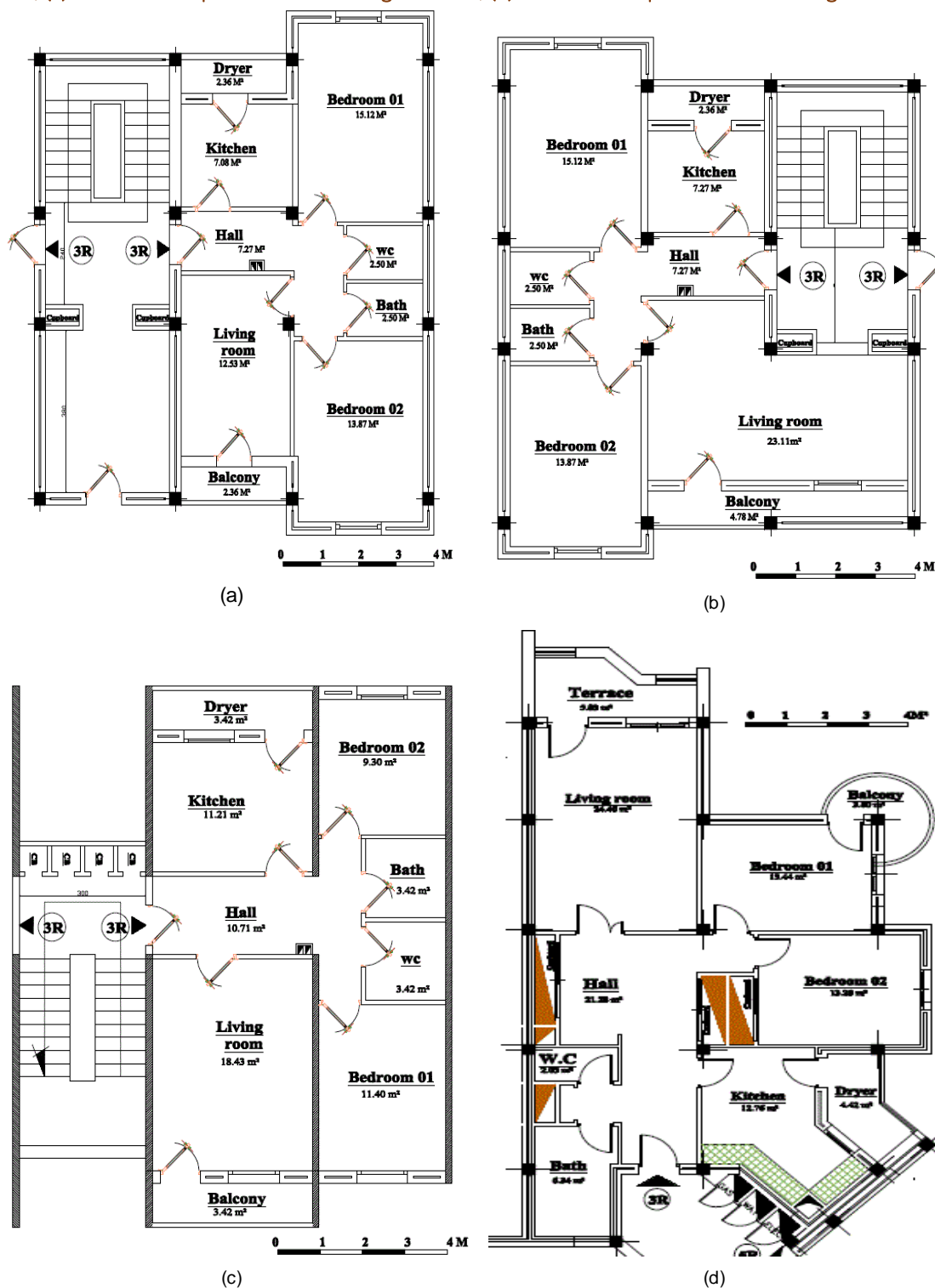
Figure 4. (a) Architectural plan of PRH housing variant 1, (b) Architectural plan of PRH housing variant 2, (c) Architectural plan of PRH housing variant 3, (d) Architectural plan of PPH housing variant 1
