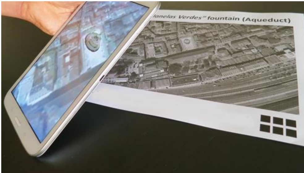
Figure 7. Using a 3D developed model in an Augmented Reality environment. The Janelas Verdes Fountain example
