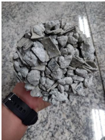
Figure 6. Pervious concrete with STT
