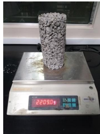
Figure 7. Pervious concrete weighing with STT
