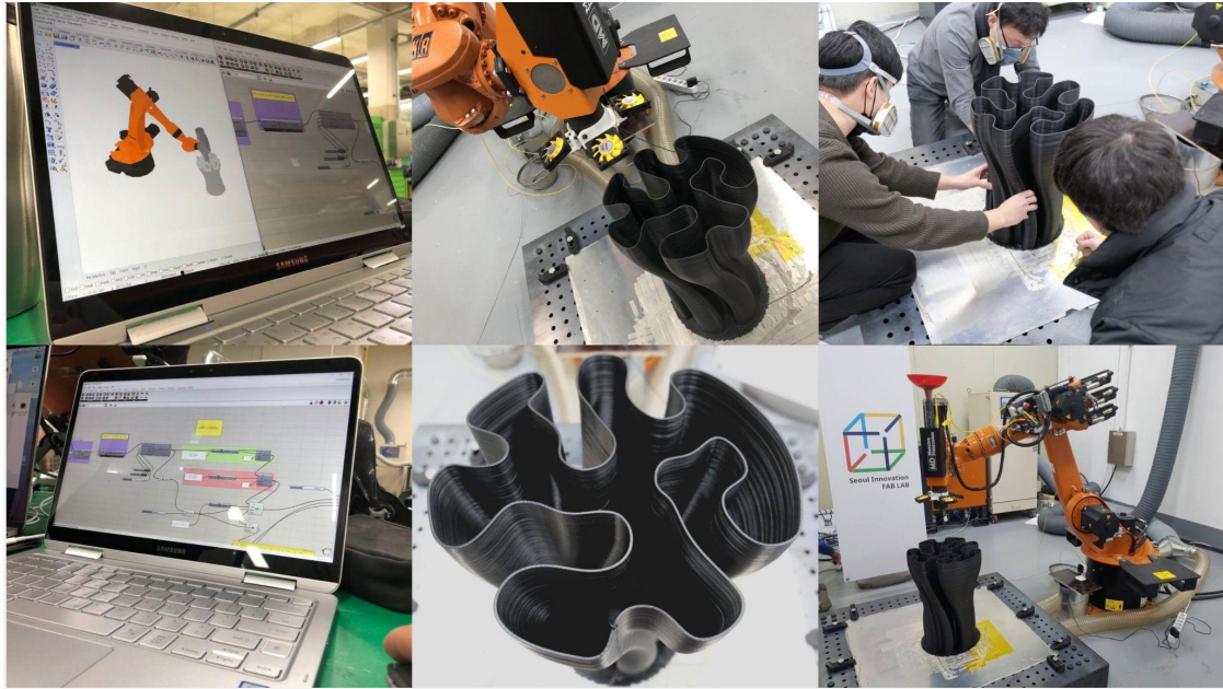
Fig. 4 Series of images showing students prototyping using Hyperconnected Hybrid model for digital fabrication of city recycled plastic
