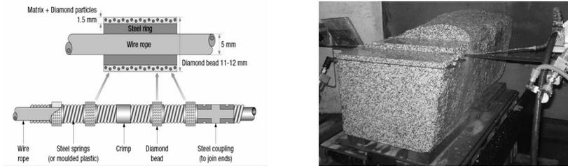
Fig. 8 Schematic view of diamond cutting wire; Fig. 9. Brown granite cutting in progress.
