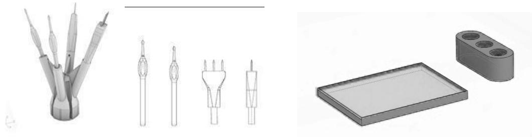
Fig. 5 Multi-device tool<sup>6</sup>: thin brush, fat brush, awl type1 and awl type 2
