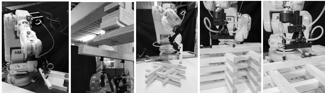
Fig. 6 Snapshots from the time-lapse of the robotic component fabrication process
