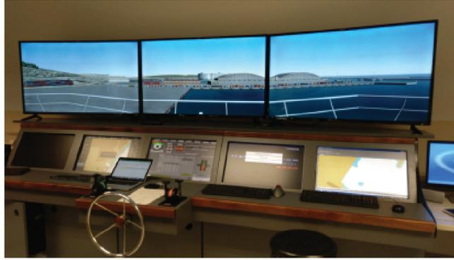
Figure 6. Picture of the bridge of the manoeuvre simulator hosted by the FNB-UPC that was used to reproduce the manoeuvres in this work (Amengual Obrador, 2019).
