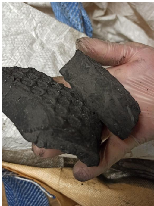
Figure 5. View of dry residue generated in a hybrid EGCS installed on board of a ship. Source: The Authors.
