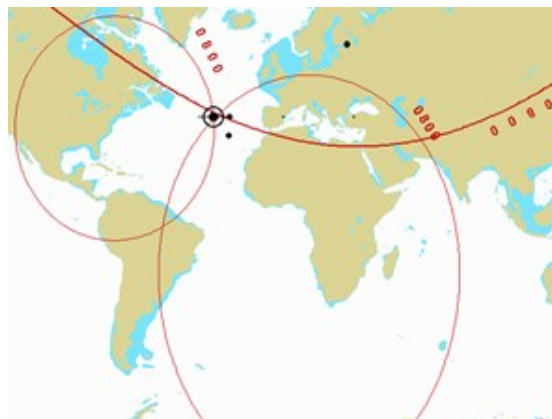
Figure 3. Fix by use of Manual Fix Position-Transas ECDIS Source: [Lušić et al, 2018]
