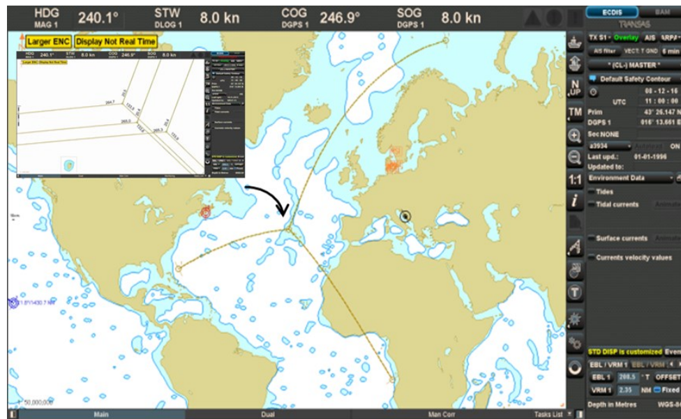
Figure 5. GP plot and use of azimuths to GP on ECDIS (Transas) to obtain fix Source: [Lušić et al, 2018]
