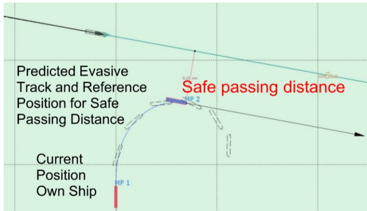
Fig. 14 Concept for „Last Line of Defence – LLoD“ for a given safe passing distance of 0.25 nm at the moment when ships are moving on parallel course: Sample for Lower Limit of manoeuvre of “Stand on Vessel” (1,3 nm)
