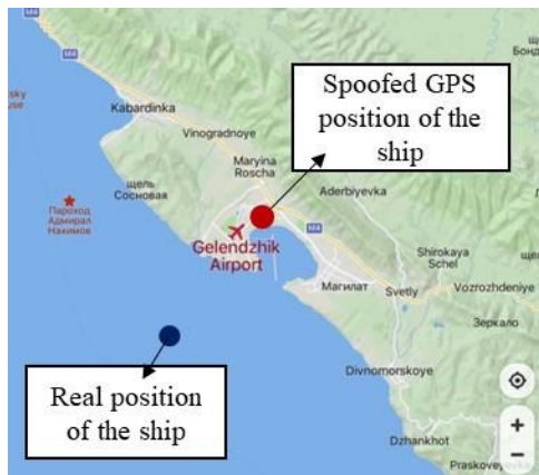
Fig. 2 The Atria tanker GPS spoofing event (adapted from [9;10])
