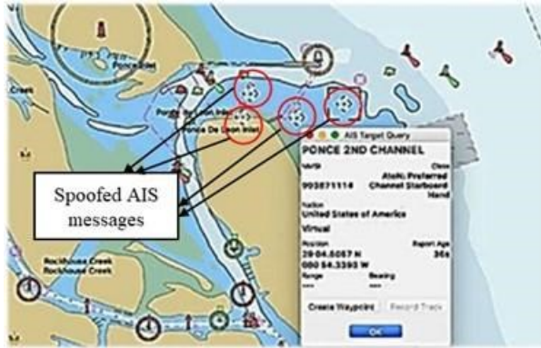
Fig. 3 Real AtoN and fake virtual AIS AtoNs (adapted from [5;11]).
