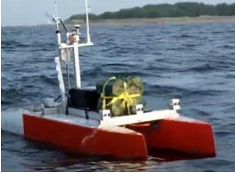
Fig. 4 Autonomous catamaran “Nymo” developed in Tallinn University of Technology [3]. The 2.5 m long vessel is of 200 kg weight class with maximal cargo limit of 100 kg and service distance of 50 km.
