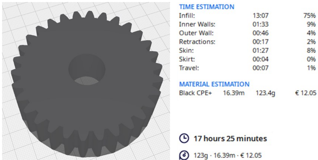
Figure 9. Preview the gear in the Ultimaker Cura before printing with CPE+
