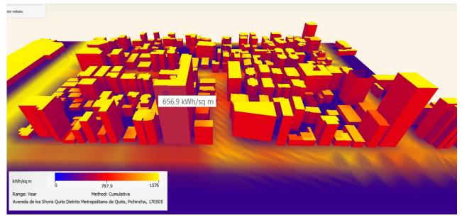
Image 11: 3d model radiation analysis high value projected scenario. Form It-Autodesk. Elaborated by authors.
