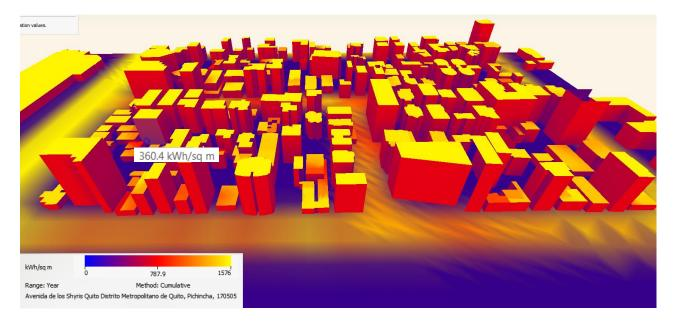
Image 07: 3d model radiation analysis low value current scenario. Form It-Autodesk. Elaborated by authors.
