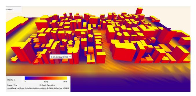
Image 06: 3d model radiation analysis high value current scenario. Form It-Autodesk. Elaborated by authors.
