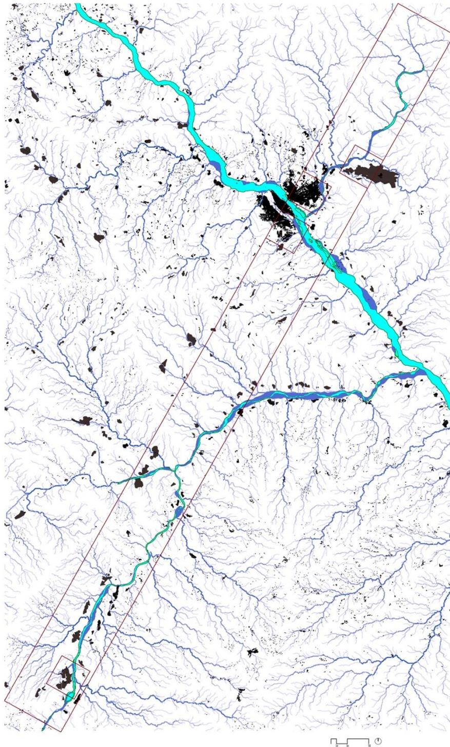
Fig. 01 River system and urbanization. Light blue is permanent water, dark blue temporary during rainy season, in black the settlements. In red the indication of the 125x10km transect and the four 5x5km cases from bottom to top: Luenha, Nhartanda, Revubue and Moatize cases, all tributary rivers of the Zambezi. Source: (Ye & Xiao, 2018, pp. 62,63)
