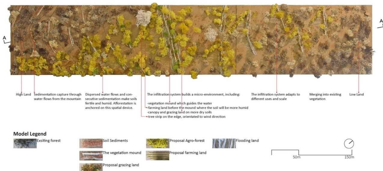
Fig. 04 The principle of cut and fill creating infiltration dams. They allow the water to infiltrate and slow down, divert and spread out over the territory as shown in the 1/500 model on the bottom. By irrigating the territory, deforested lands regain their vegetation and some agricultural practices can exist. Source:Project by Xiao Xinyu. (Xiao, 2018, p. 60)
