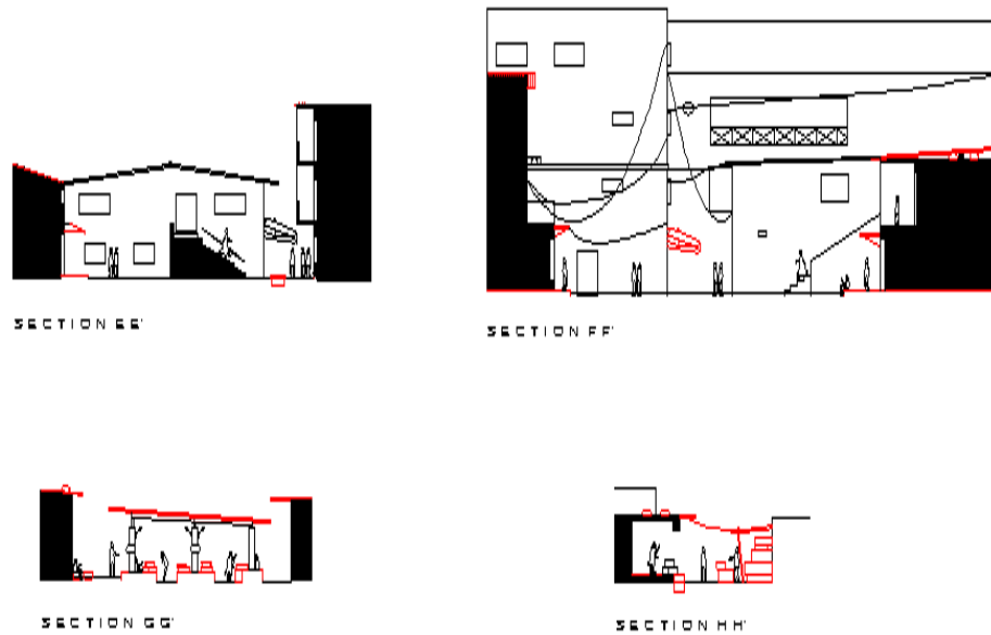
Fig. 06 Plans and cross-sections derived from the neighbourhood of Koliwada in Dharavi (Author). Red: Indigenous built elements.
